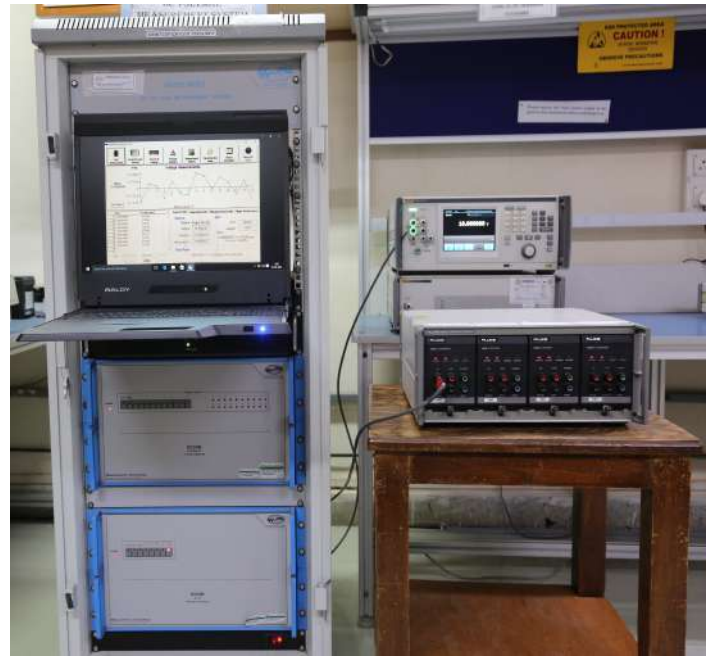
Calibration of DC Voltage by using Binary Voltage Divider
