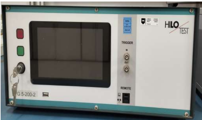
Telecom Surge Generator
