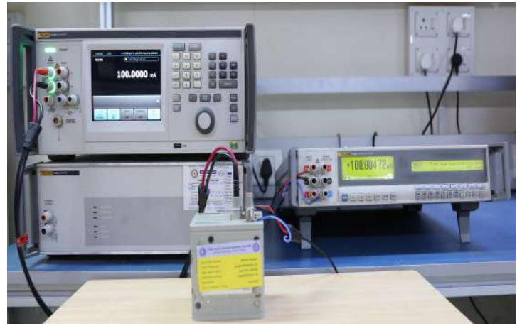
Calibration of DC Current By using Standard Resistor
