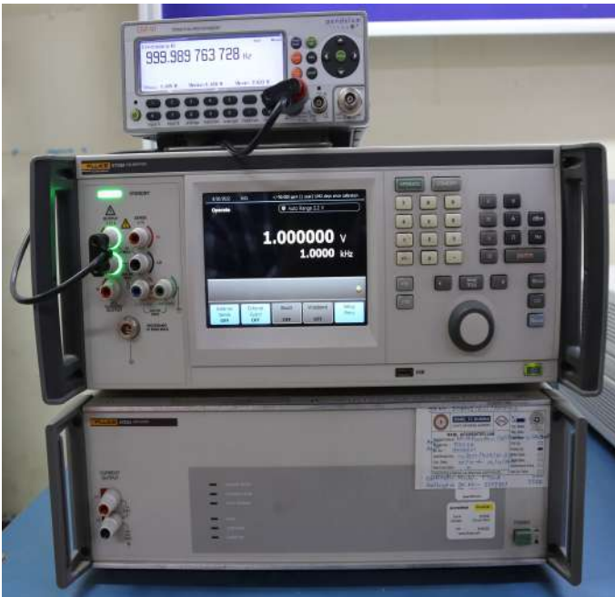
Calibration of Frequency by using Oven Controlled Crystal Oscillator
